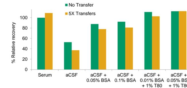
Figure 4. Relative recovery of ASO1 in different aCSF proxy solutions following 5x transfer test in LoBind tubes at low QC level (1.50 ng/mL)
