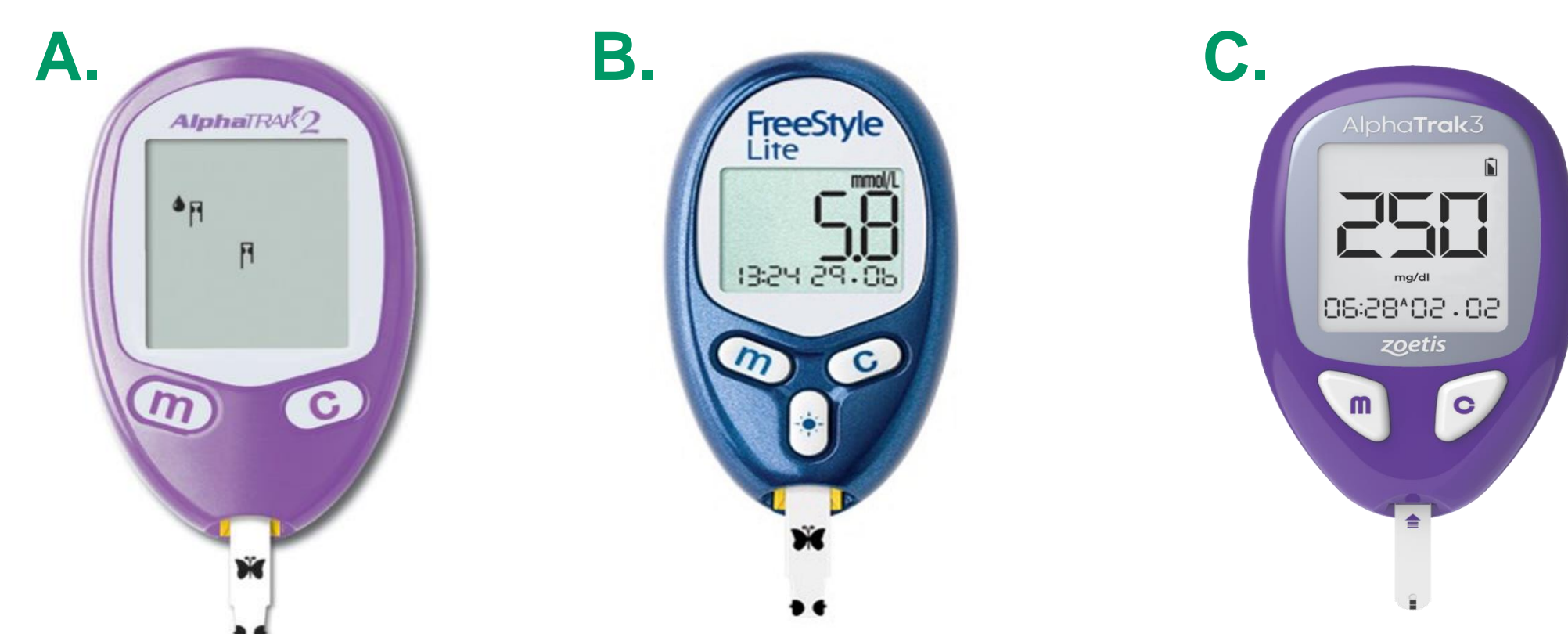
Figure 1. Glucometers evaluated in Preliminary Trial. 1A) AlphaTrak 2 – Veterinary glucometer historically used at our facility but commercially discontinued. 1B) FreeStyle Lite – a human glucometer. 1C) AlphaTrak 3 – Veterinary glucometer marketed for dogs & cats. Both codes were evaluated.
