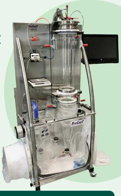
Spray drying can enable poorly soluble compounds to become viable drug products, even in cases where no clear path forward previously existed. As over 70% of New Chemical Entities (NCEs) are considered poorly soluble, spray drying offers a path forward for these otherwise abandoned molecules and allows them a chance to become marketed drugs.
